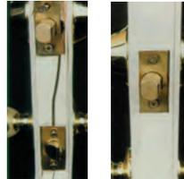
The unequalled security of steel - A wood edge steel door (left) cracked under the force of one hit of a 100 lb. test weight. Steel edge doors (right) did not force open after seven hits of a 100 lb. test weight.
