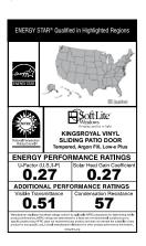
Double-Pane insulated tempered glass with Argon Gas, Intercept<sup>®</sup> spacer and Solar Low-E
